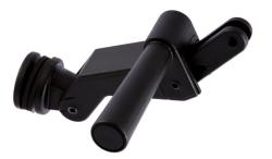
This easy to operate window hold-open is designed to fit comfortably in the hand for top and side hinged venting windows for on– and off-highway vehicles. It features an over center design that orientates the window at fully closed and fully open positions and an optional quick release pin in bright red nylon or steel.
